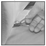
1. Reach over the second row seat and pull up on the strap loop. Then pull the seat cushion up and push it forward.
